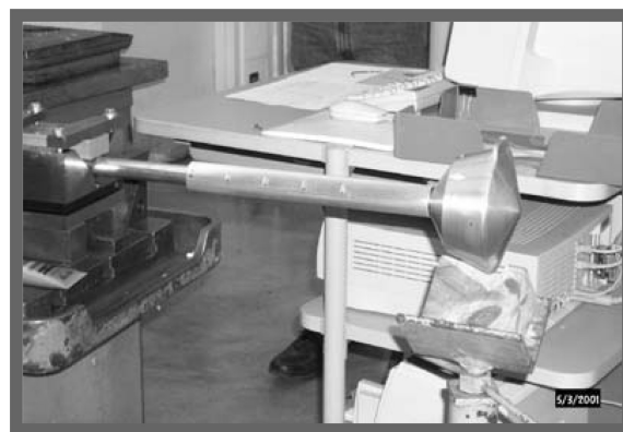
Fig. 3 Photograph of wind-tunnel model with balance shroud.
