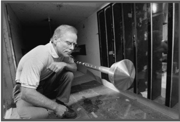
Fig. 4a Installation of Mars Smart Lander baseline model in the UPWT at LaRC.
